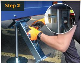
Position Support Stands to all four hydraulic rams and secure using sword pins attached.
