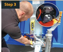
Remove hydraulic power pack lead from socket under nosecone. (Advised for Health & Safety).
