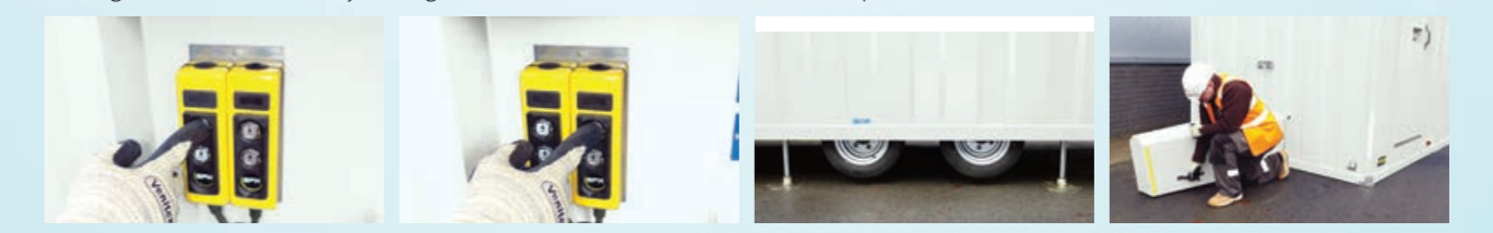
Push button controls to lower front and rear hydraulic rams
