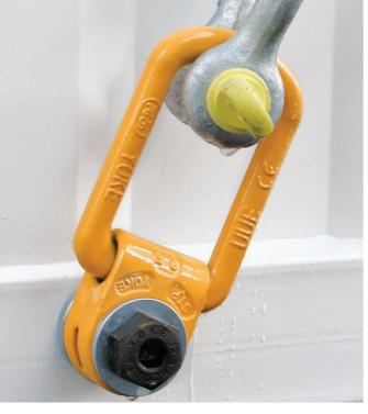
**NOTE:** When using yoke type screw-in lifting eyes, ensure that they are secured prior to liftir
