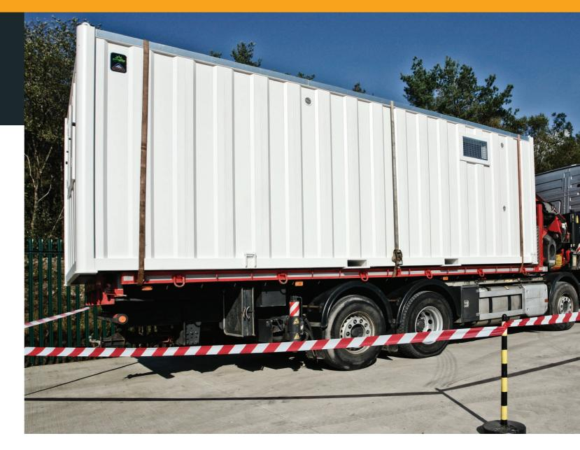
When securing static unit to flatbed lorry, we recommend using a minimum of 3 straps.
