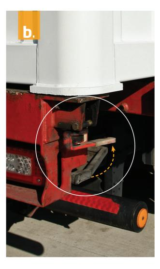
**NOTE:** If lorry is not equipped with twist-locks, then ratchet straps over the unit will be required to secure the load.
