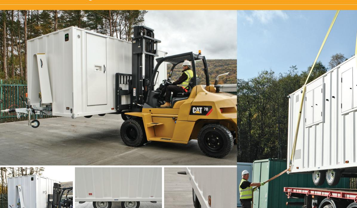
• Ensure the fork lift truck has the safe lift capacity:
