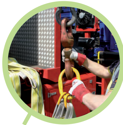
2 Attach Flat Webbing Sling to HIAB lifting hook
