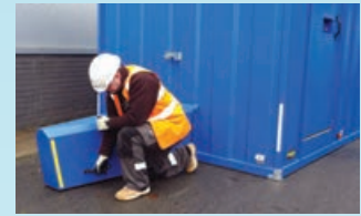
Unit is lowered and canopy locked to protect towing facility
