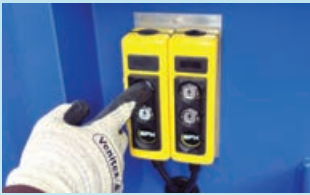
Push button controls to lower front and rear hydraulic rams
