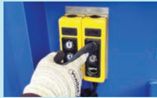
Push button controls to lower front and rear hydraulic rams
