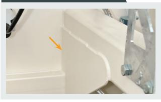
Ensure breakaway cable is fitted and free of damage.
