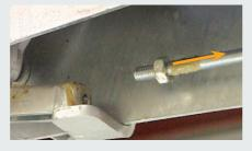
Remove two M16x135 coupling bolts from towing coupling – the coupling will then fall away
