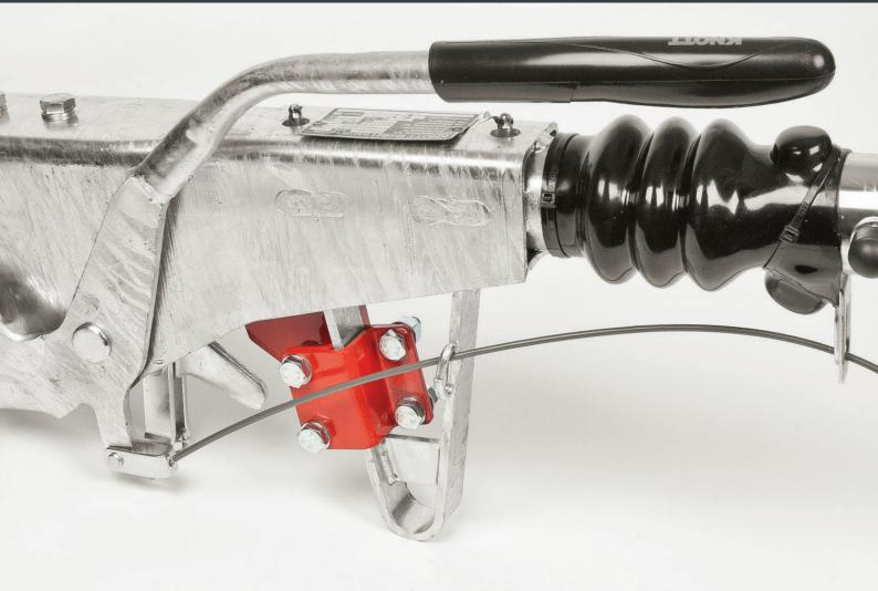
How to fit the Handbrake Protection Skid Strengthening Bracket
