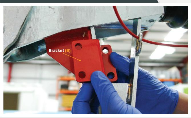
Insert 10mm bolts and washers through strengthening bracket holes.
